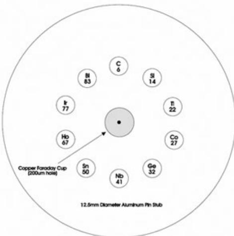
**Purpose of standard:** Calibration and testing of energy-dispersive X-ray systems and backscattered electron detectors.
